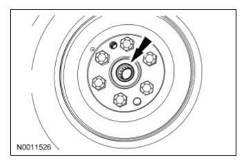
Install the clutch disc and the clutch pressure plate. For additional information, refer to <u>Clutch Disc and Pressure Plate — 4.6L</u> or <u>Clutch Disc and Pressure Plate — 5.4L</u> or <u>Clutch Disc and Pressure Plate — 5.4L</u> in this section.
